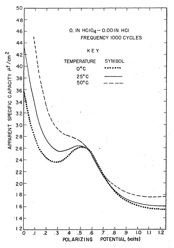
function of the temperature. The polarizing potential is referred to the potential of the silver-silver chloride reference electrode at 25° C. as explained above.
