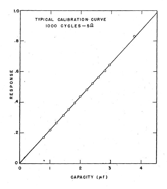
illustrates the linearity of the response of the instrument to varying capacity in the circuit.
