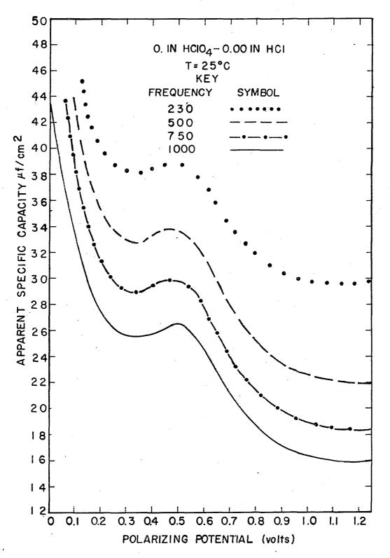
Figure 11. Apparent specific capacity of the electrical double layer on mercury in 0.1N perchloric acid versus polarizing potential for several operating frequencies at 50° C.
